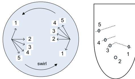
Fig. 4. Fuel valve and nozzle holes arrangement
