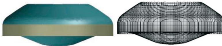
Fig.3. Combustion chamber model and mesh domain at firing position
