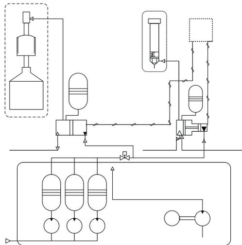
Fig. 1. Outline of the ME engine fuel oil injection system
