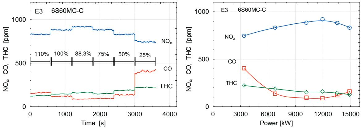
Fig. 5. Measured raw exhaust gas emission component profile of 6S60MC-C engine
