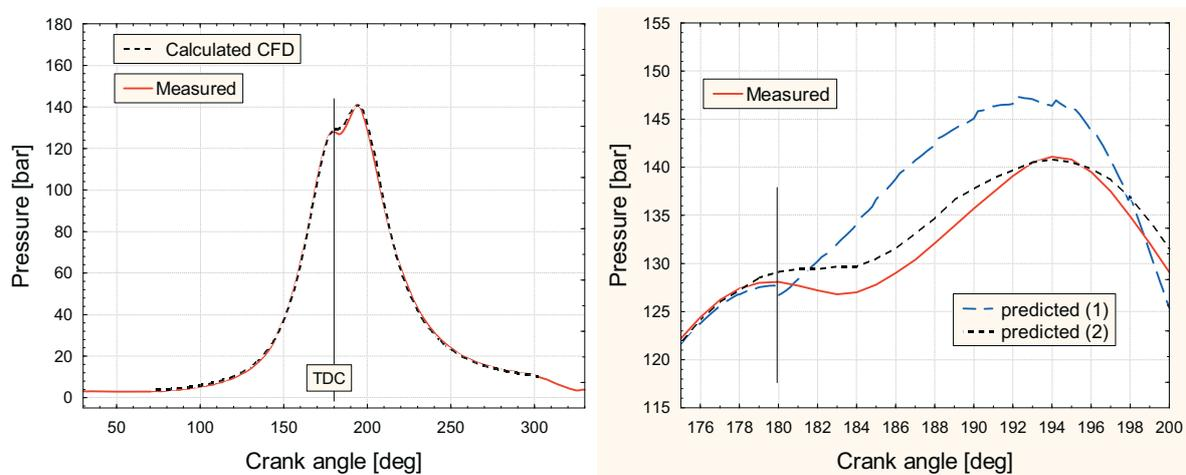
Fig. 8. Comparison of calculated and measured cylinder pressure under 100% effective load
