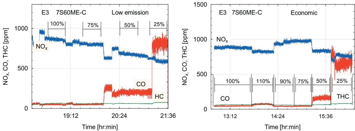
Fig. 6. Measured raw exhaust gas emission component profile of 7S60ME-C engine in low emission and economic mode
