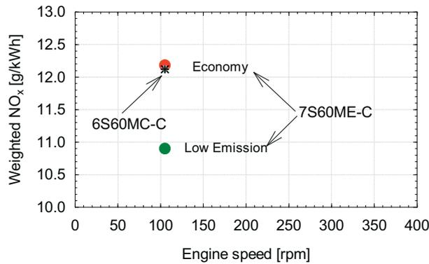
Fig. 11. The total weighted NO<sub>x</sub> emission factor of 6S60MC-C and 7S60ME-C engines
