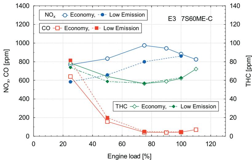
Fig. 7. Average emission component profile comparison of 7S60ME-C engine in two modes of operation
